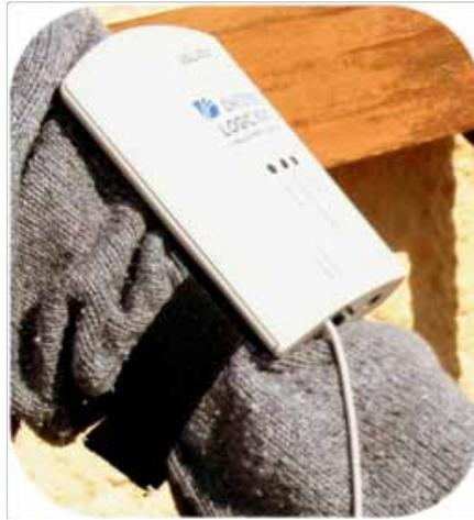
View of the RFID reader, portable computer and thumb cover with integrated antenna
