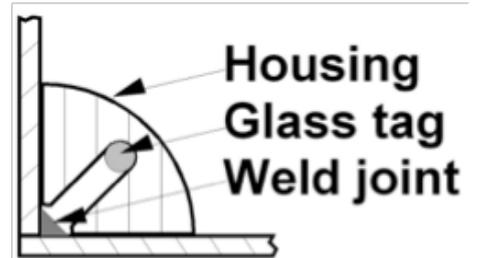
least two steel parts welded at 90° to each other, we designed a tag housing to be mounted directly on the weld joint. Inside we used a glass tag. The housing with tag was mounted using hot-melt adhesive. The housing was placed close to some corner, where it was optimally protected, even when the parts were thrown down into the box.
