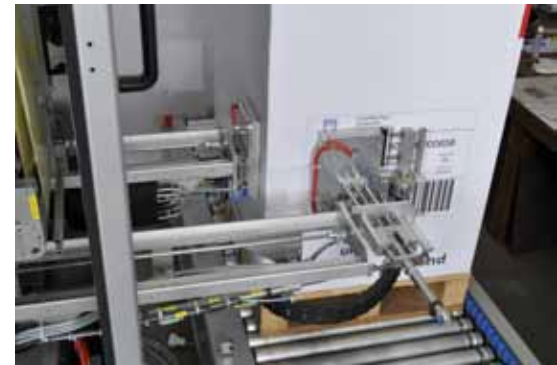
Logopak system with two labeling arms and integrated RFID transponder. – Photo: Logopak Systeme
