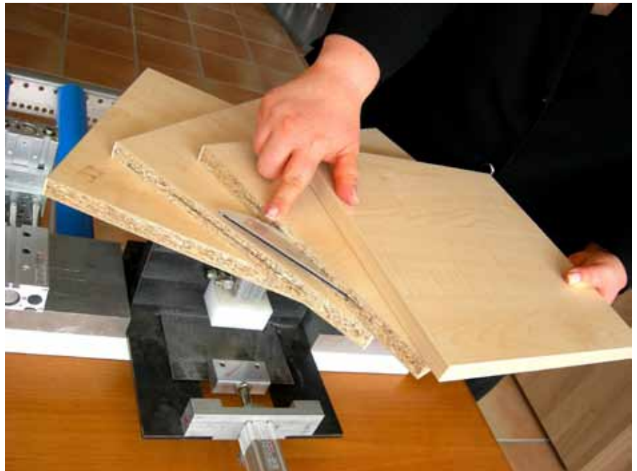
Ready for use over the entire supply chain: the Abatag is inserted into a special slot machined in the panel in the CNC machining center and then encapsulated. This ensures that the RFID chip is present and protected during the entire product lifetime. – Photo: abaco
